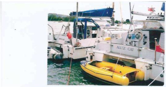
Two types of davits both with similar fixings. Both light in weight. The boat on the right the davit mounts are stronger being supported by both the bathing platform and wooden blocks c/o Brighton Marina another advantage being the dinghy weight rests not only on the rear lockers but on the platform also.
